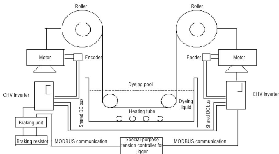
Schematic Diagram of Dual-Inverter Control in Jigger
